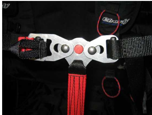
The chest strap correctly closed
