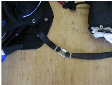
Connection using screw-lock link
