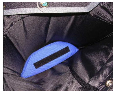
Container with spacer Important : Fleece towards the reserve !!!
