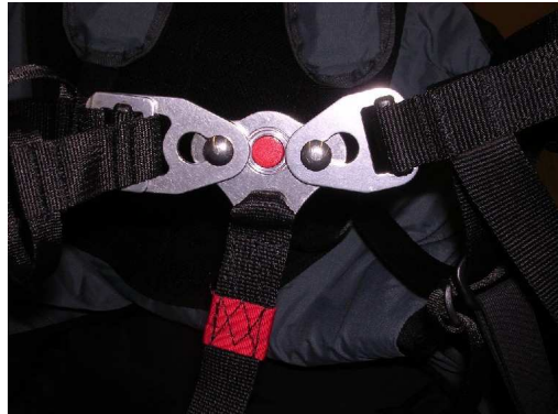
The properly closed chest strap
