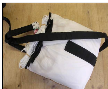
Connection harness strap / bridle line
