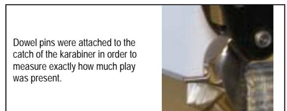
To approximately test the safety of a karabiner every pilot can establish the point of actuation by gravity  $F_k$  of his karabiner for himself by measuring the loading required up to the point where the catch can no longer be opened.
